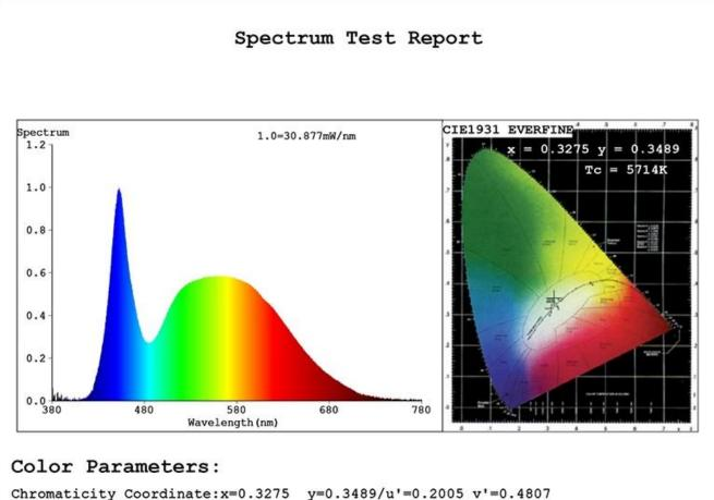
Tc=5714K Dominant WL:Ld =530.1nm Purity=3.3% Red Ratio:R=15.2% Peak WL:Lp=452.4nm HWL:Lhd=26.6nm Render Index:Ra=82.1 R1 =79 R2 =87 R3 =92 R4 =81 R5 =80 R6 =82 R7 =88 R10=68 R11=79 R8 =68 R9 =5 R12=57 R13=81 R14=96 R15=74 Photo Parameters: Flux = 1291 lm Eff. : 68.67 lm/W Fe = 4.019 W Electrical parameters: V = 230.0 VI = 0.08500 A P = 18.80 W PF = 0.9630 LEVEL:OUT WHITE:OUT
