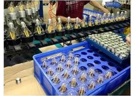
Automatic Base Mounting Line
